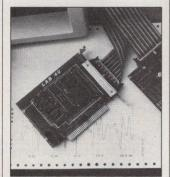
LAB 40, an input/output bus for data acquisition and control
